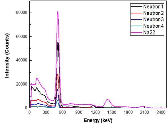
Fig. 3. The measured energy spectrum of the activated Cu-62  $t_d$  (elapsed time after irradiation) of a Neutron 1 through 4 were 7 min., 11 min., 20 min., 34 min., respectively.
