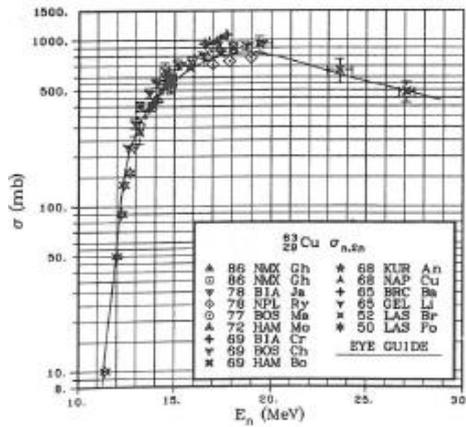
Fig. 3. Cross-section of Cu-63 with respect to neutron energy. [2]
