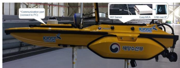
Fig 1. Overall configuration of the in-situ oceanic radiation monitoring system.
