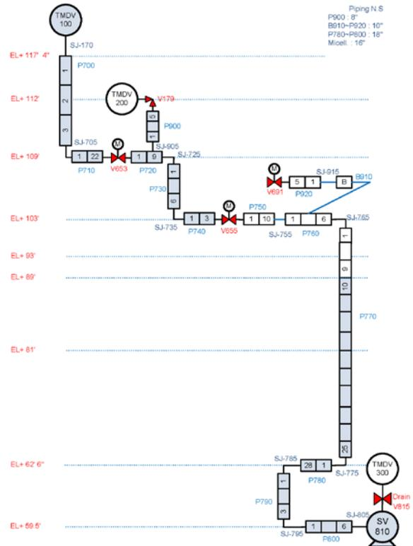
Fig. 1. Nodding diagram for RELAP5
