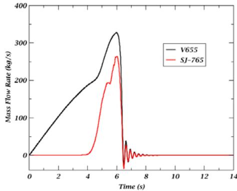
Fig. 6. Mass flow behaviors at isolation valve (V-655) and piping (SJ-765)
