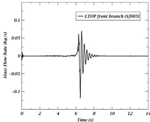
Fig. 7. Mass flow behavior at branch junction (SJ905) to the LTOP valve
