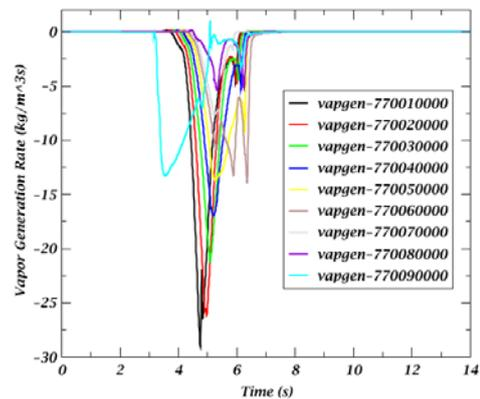
Fig. 5. Vapor condensation behaviors in vertical pipe (P770)
