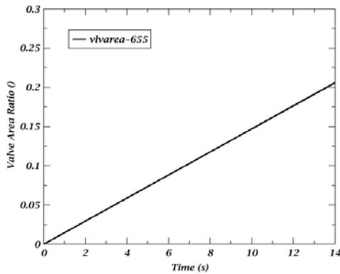
Fig. 3. Valve (V-655) opening rate
