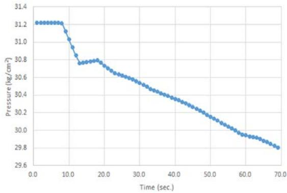
Fig. 2. Measured data for Pressurizer pressure
