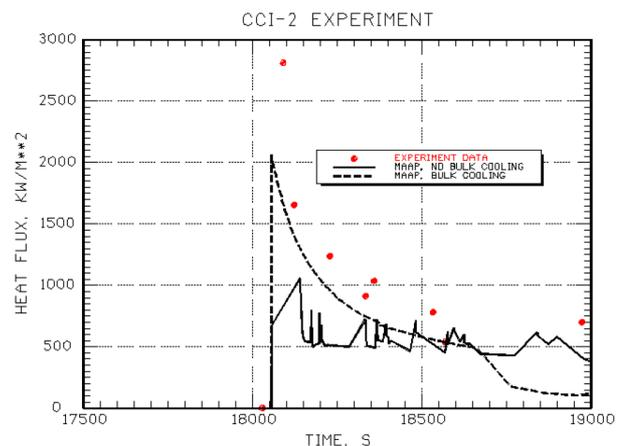
Fig. 1. Comparison between MAAP Calculated Heat Flux with Bulk Cooling Model On/Off and CCI-2 Data [1]
