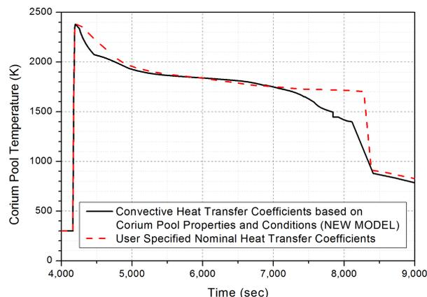
Fig. 5. Comparison of Corium Pool Temperature according to Heat Transfer Correlations Options
