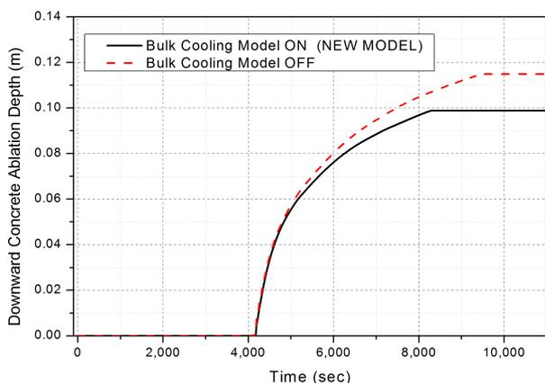
Fig. 4. Comparison of Downward Concrete Ablation Depth according to Bulk Cooling Effect
