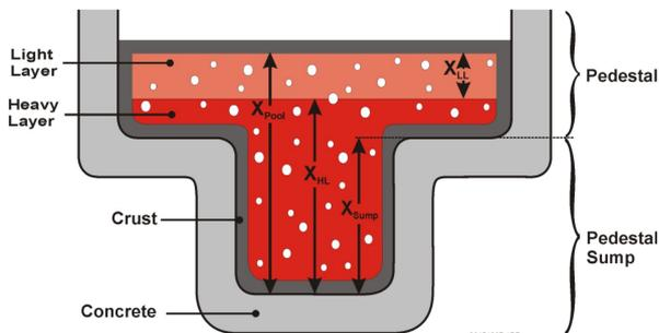
Fig. 2. Stratified Ex-Vessel Corium Pool [1]
