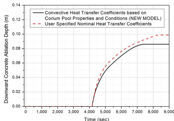
Fig. 6. Comparison of Downward Concrete Ablation Depth according to Heat Transfer Correlations Options
