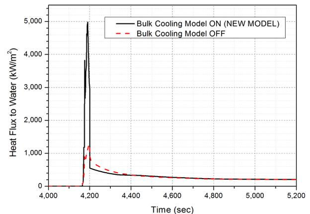
Fig. 3. Comparison of Heat Flux to Water according to Bulk Cooling Effect
