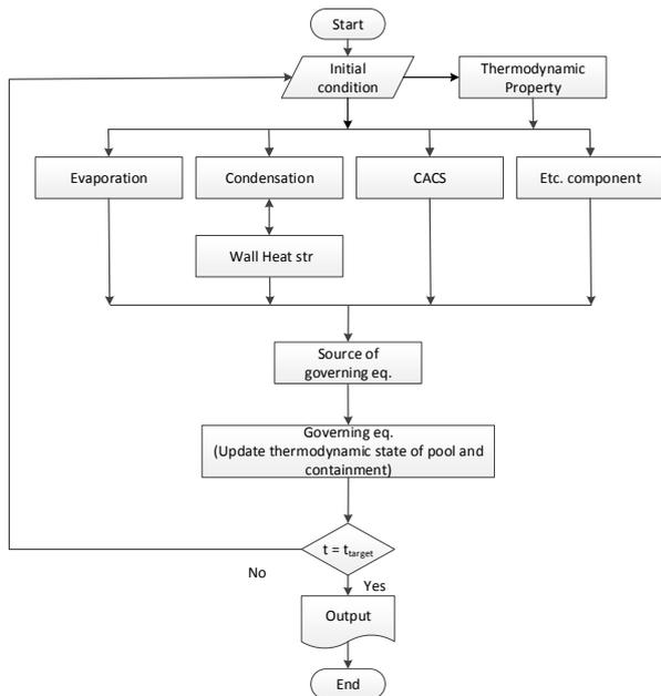
**Fig. 2. Structure and logic of code**
