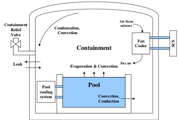
**Fig. 1. Schematic of calculation region and phenomena**
