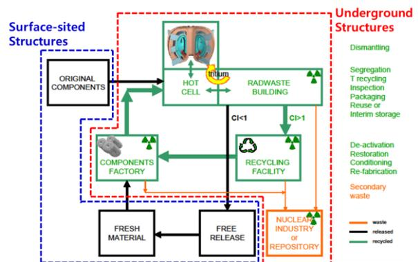
Fig. 3. Diagram of recycling and clearance processes through the closed cycle of fusion power material for fusion reactor structure located in the underground and surface-air sites.
