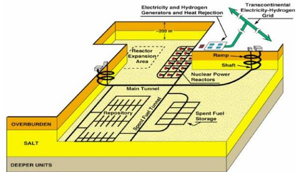
Fig. 1. Concept of an UNP in a shallow and massive salt deposit [2].
