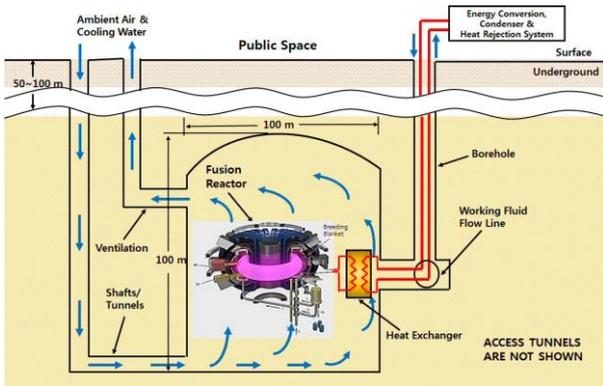
Fig. 2. Schematic of underground nuclear reactor, reactor chamber, ventilation system, and working fluid transfer system.
