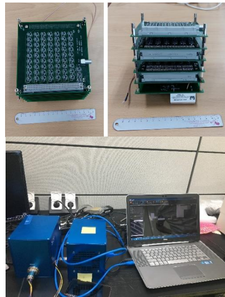
Fig. 1. The photographs of developed low noise DAQ system without HV module (top) and with AI case and imaging software (bottom).
