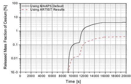
Fig. 5. The released mass fraction of Cesium in the unmitigated sequence.
