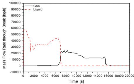
Fig. 3. The mass flow rate through the SG tube break in the unmitigated sequence.
