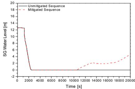
Fig. 4. The water level of the faulted SG.
