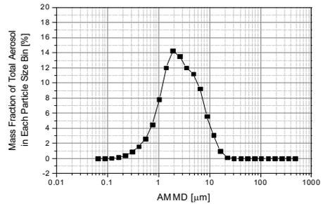
Fig. 6. The particle size distribution calculated by the MAAP5 at 10,000 seconds
