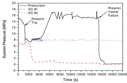
Fig. 2. The RCS and the SG pressure in the unmitigated sequence.
