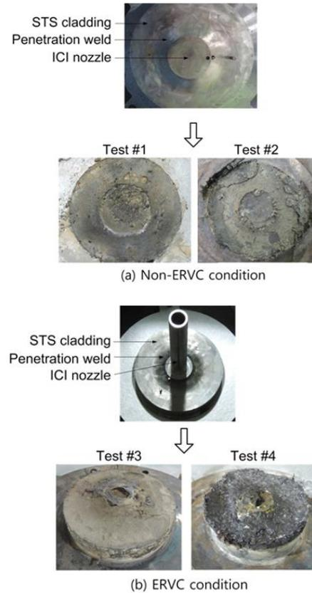
Fig. 4. Photos of test specimen before and after the experiment
