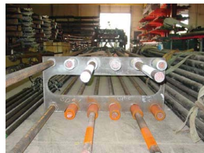
Fig. 7. Template for rebar placing [6].
