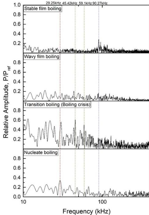
Fig. 7. Power spectrum density of vapor-liquid interface wave in different boiling regimes
