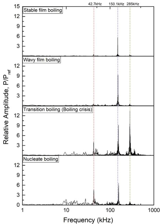
Fig. 5. Power spectrum density of AE signals in different boiling regimes
