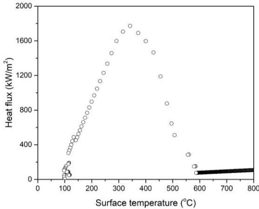
Fig. 2. Boiling curve by inverse heat transfer method
