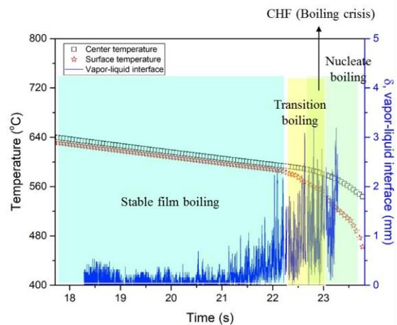
Fig. 6. Plot of vapor-liquid interface position with the time
