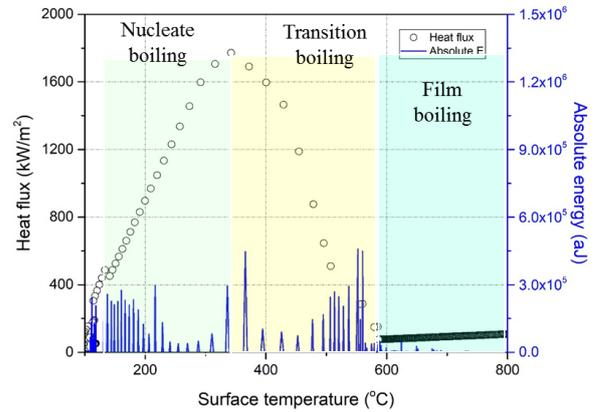
Fig. 3. AE absolute energy with boiling curve
