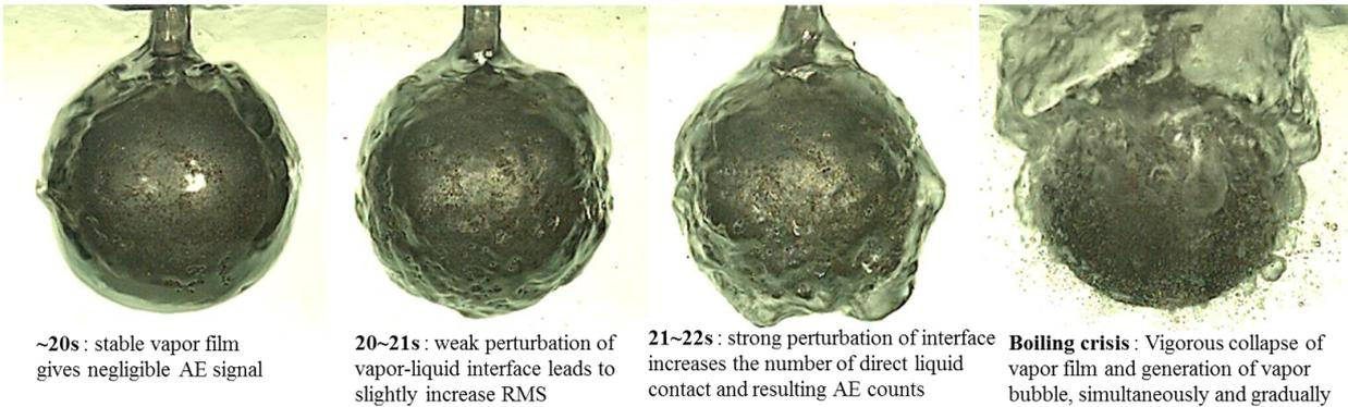
Fig. 4. Representative images of test section during each time period in AE absolute energy plot
