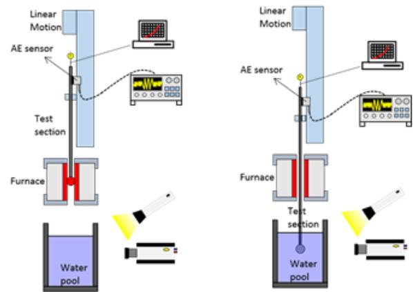
Fig. 1. The schematic diagram of experimental facility with AE sensor and high-speed camera.
