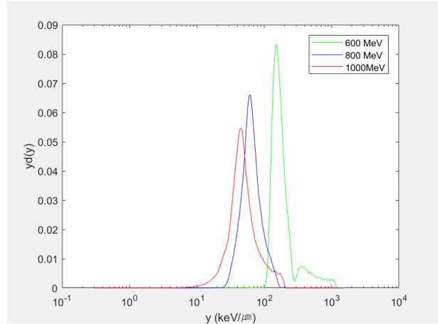
Fig. 4.  $yd(y)$  spectrum of carbon-12 ion in 5 mm Perspex phantom. Energy of the ion is changed from 600 MeV/u to 1000 MeV/u
