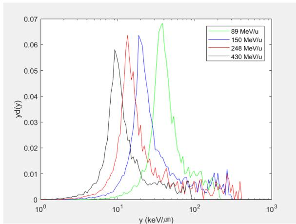
Fig. 3.  $yd(y)$  spectrum of carbon-12 ion in 5 mm Perspex phantom. Energy of the ion is changed from 89 MeV/u to 430 MeV/u
