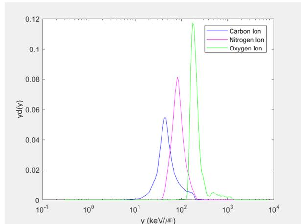
Fig. 5.  $yd(y)$  spectrum of carbon, nitrogen, and oxygen ion. Particle energy was set to 1000 MeV/u
