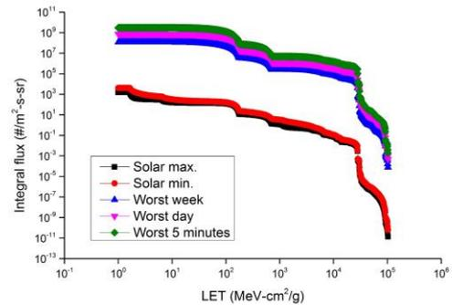
Fig. 1. LET-flux spectra of GCR environment, CREME96 model.
