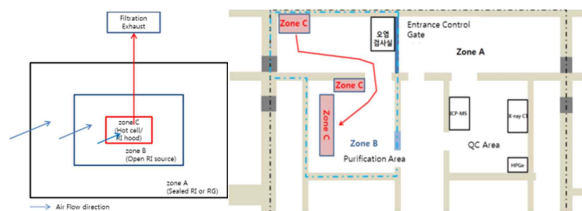
Fig. 4. Purification area for RI production
