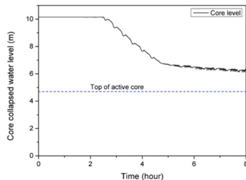
Fig. 4. Core collapsed water level (Phase 1)
