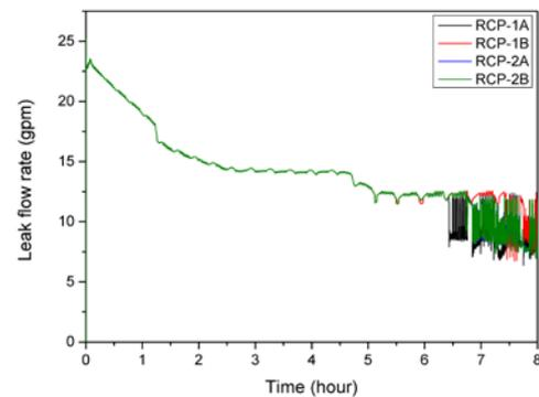
Fig. 3. Flow rate of RCP seal leak (Phase 1)
