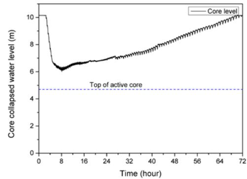
Fig. 7. Core collapsed water level (Phase 1 and Phase 2)
