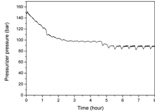
Fig. 2. Pressurizer pressure (Phase 1)
