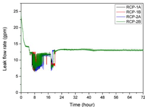
Fig. 6. Flow rate of RCP seal leak (Phase 1 and Phase 2)
