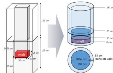
Fig 3. Scaling analysis for geometry (CCI-3): experiment (left), and MELCOR (right)
