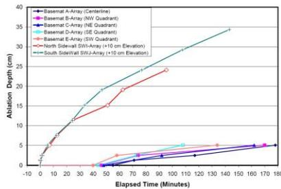
Fig. 2. Maximum axial/radial ablation depth (CCI-3)
