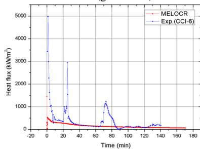
Fig. 9. Heat flux between corium and water of CCI-6: experimental data (blue dot); case 17 (red line)
