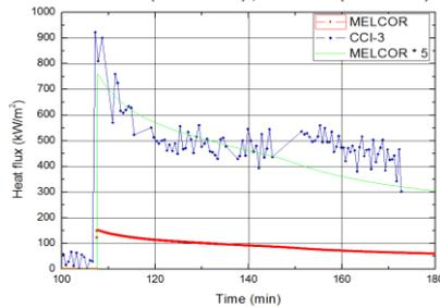
Fig. 8. Heat flux between corium and water of CCI-3: experimental data (blue dot); case 17 (red line); five times of case 17 (green line)
