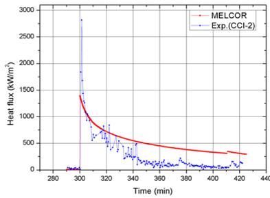
Fig. 7. Heat flux between corium and water of CCI-2: experimental data (blue dot); case 8 (red line)
