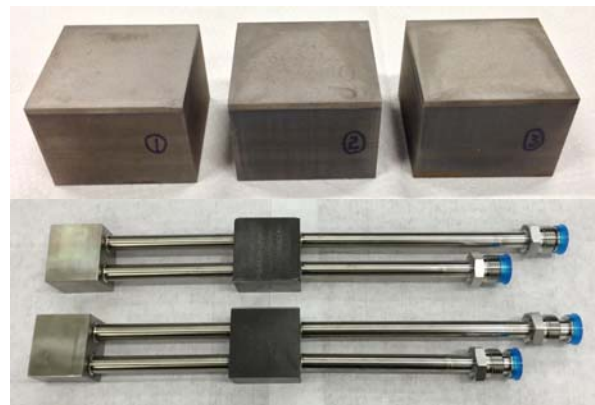
Fig. 2. W/FMS HIP bonding mockups (top) and coated mockups (bottom).
