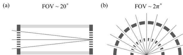
Fig. 1. Field of view (FOV) of RMC: (a) conventional design and (b) H-RMC.
