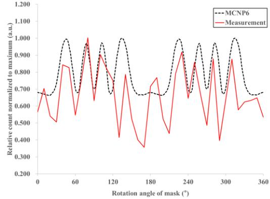
Fig. 4. Comparison of modulation patterns obtained by measurement and MCNP6 at  $(r, \theta, \varphi) = (25 \text{ cm}, 30^\circ, 180^\circ)$ .
