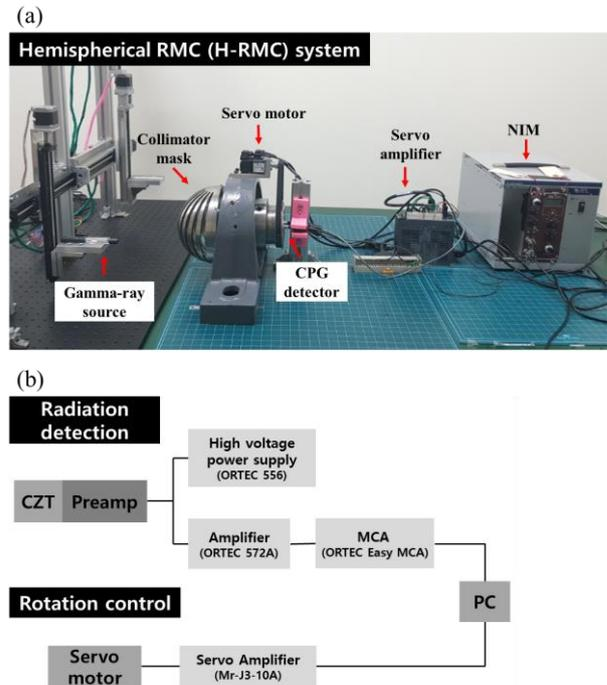
Fig. 2. (a) H-RMC system and (b) block diagram of radiation detection/rotation control system.
