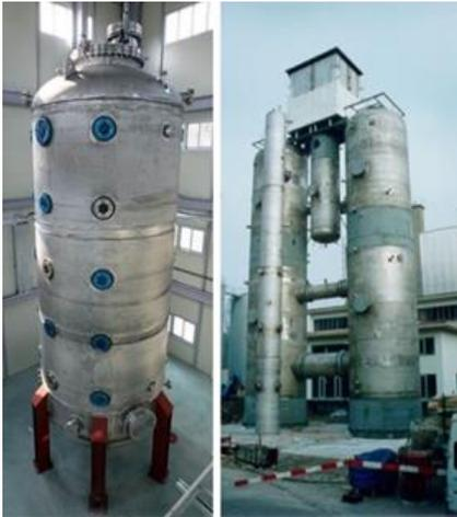
Fig. 2. Test vessels: SPARC (left), and PANDA (right).
