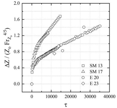
Fig. 3. Comparison of experimental database of SPARC and PANDA on stratification erosion.
