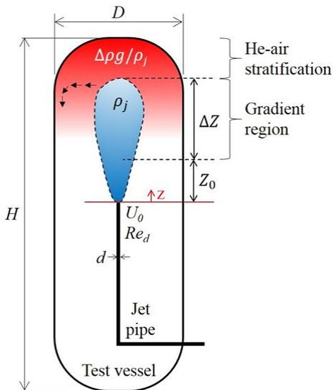
Fig. 1. General test on stratification erosion.
