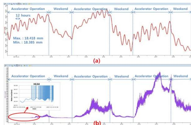
Fig.3. Variation in water level of two HLSs for 3 weeks: (a) HLS1 located in end of accelerator tunnel, (b) HLS4 located in 100 MeV beam-dump with abnormal signal.
