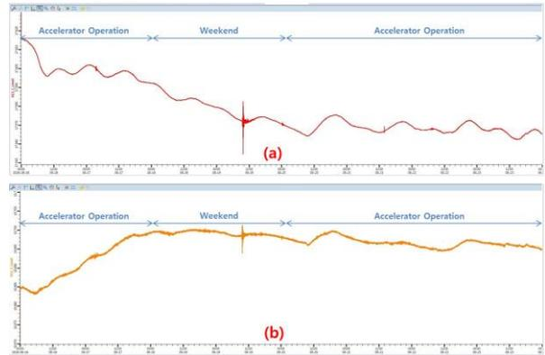
Fig.6. Tendency of water level after modified of HLS electronics layout: (a) HLS1, (b) HLS5
