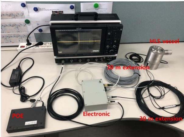
Fig.4. Test of Extended cable
