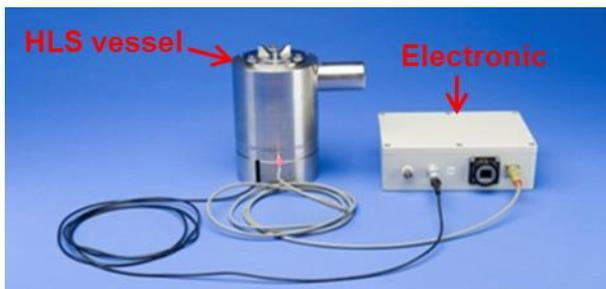
Fig.1. Hydrostatic Leveling System
