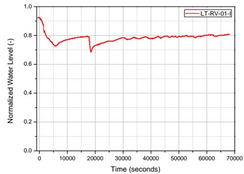
Fig. 2. Collapsed Water Level of Reactor Pressure Vessel.
