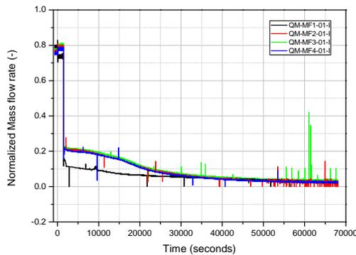
Fig. 5. Flow Rate of Secondary System (PRHRS).
