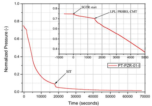
Fig. 1 Pressurizer Pressure in the Reactor Coolant System.
