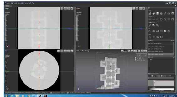
Fig. 8. Radiographic images taken by developed system
