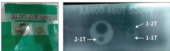
Fig. 7. Hole-type indicators and radiographic image
