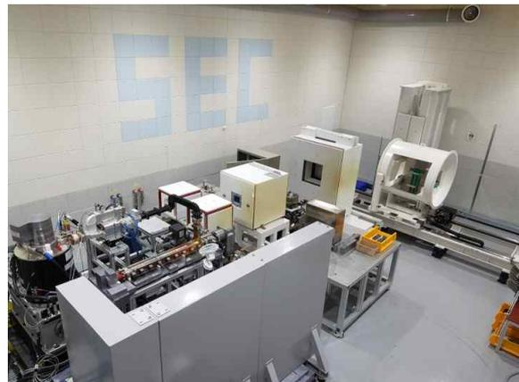
Fig. 3. Developed high energy X-ray inspection system
