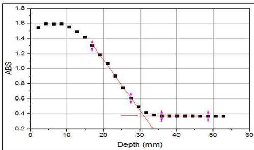
Fig. 6. E-beam energy measurement by ASTM 51649 standard
