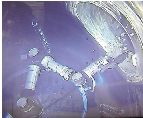
Fig.6. The AUroRA Scanning the Nozzle to Pipe under the water on Shinhanul unit 2
