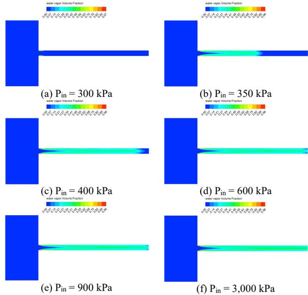
Fig. 4. Distribution of vapor volume fraction depending on the different upstream pressures.
