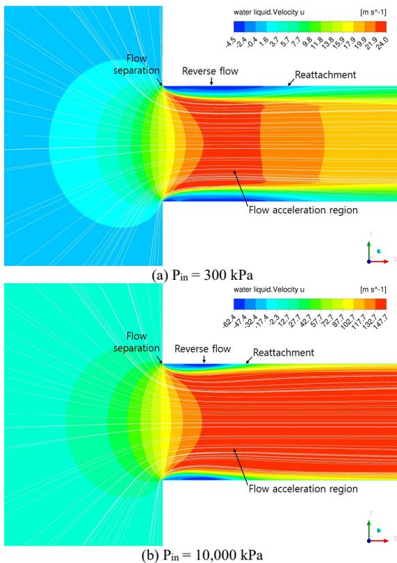
Fig. 3. Distribution of axial velocity and streamlines at the different upstream pressures.
