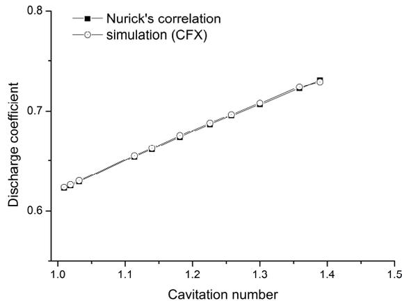
Fig. 6. Comparison of the predicted discharge coefficients  $C_d$  and Nurick's correlation.
