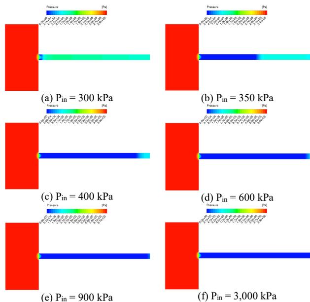
Fig. 5. Distribution of static pressure depending on the different upstream pressures.
