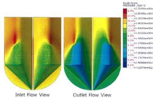
Fig. 1 Pressure distribution under normal flow condition with 50% clogged
