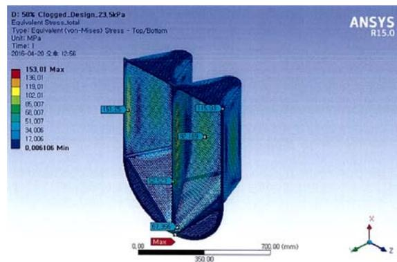
Fig. 2. Distribution of equivalent stress under design flow condition with 50% clogged
