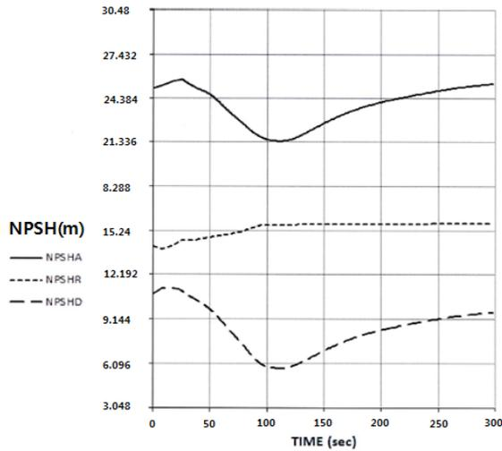
Fig. 3 Comparison of NPSHav and NPSHre under the transient condition of turbine trip
