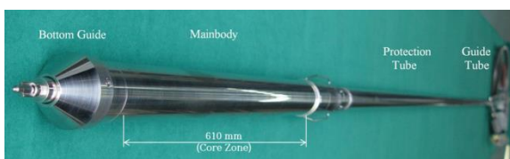
Fig. 1. Instrumented capsule for the material irradiation test
