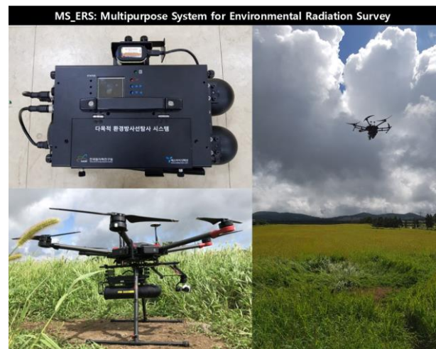
Fig. 1. The multipurpose system for environmental radiation survey and its application to the airborne survey
