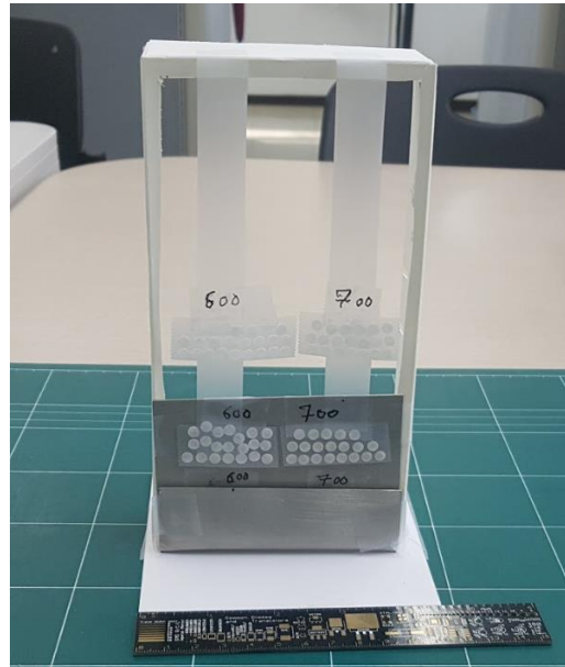
Backward view of the TLD setup with cadmium sheet in place
