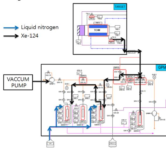
Fig. 2-2 Recovery path of high purity xenon gas
