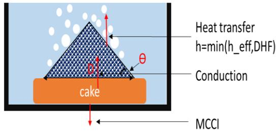
Fig. 2. Heat transfer in the debris bed and cake
