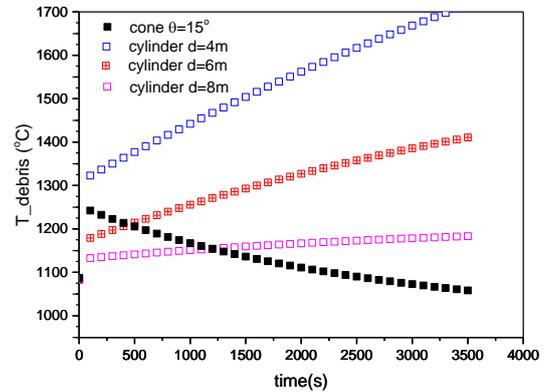
Fig. 3. Debris bed temperature with various shape
