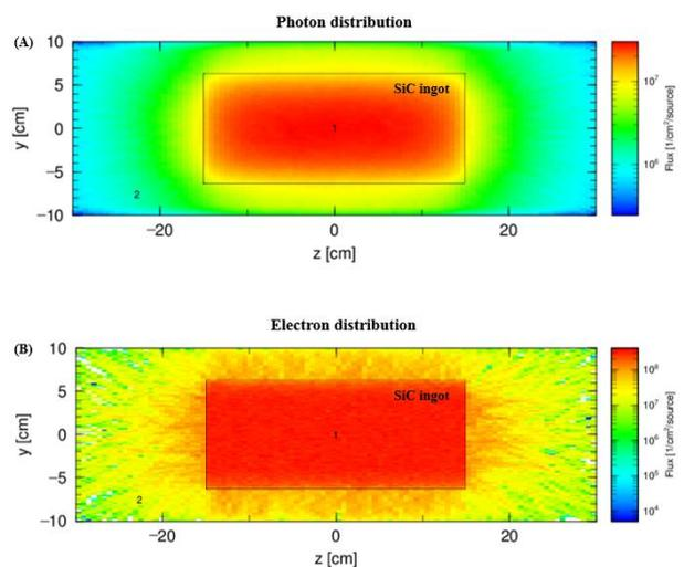
Fig. 1. Distribution of (A) gamma-rays and (B) electrons emitted from the irradiated SiC viewed in y-z plane (plotted by ANGEL 4.50).
