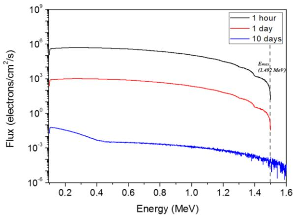
Fig. 2. Energy spectra of electrons in the SiC volume at 1 hour, 1 day and 10 days after neutron irradiation.
