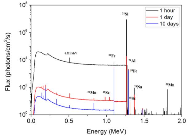
Fig. 3. Energy spectra of gamma-rays (photons) in the SiC volume at 1 hour, 1 day and 10 days after neutron irradiation.
