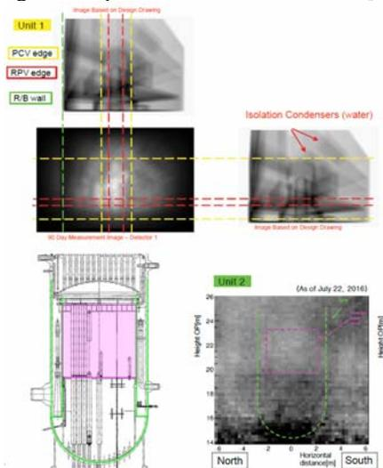
Fig.2 Status of Molten Core for unit 1 and 2[3]
