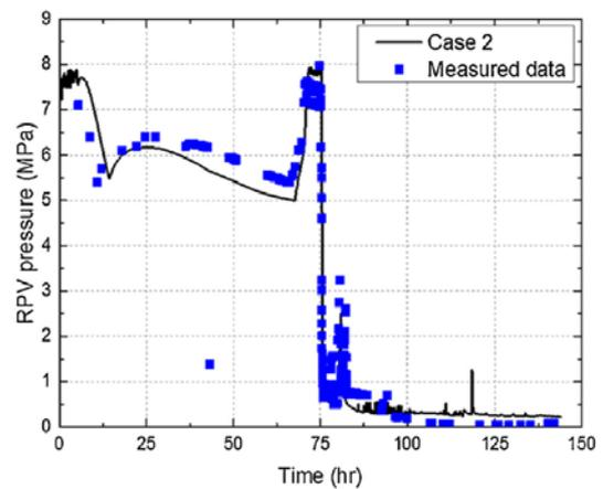
Fig.1 RPV pressure for FDNPP unit 1 [2]
