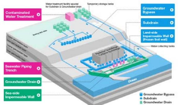
Fig.7 Measures for the isolation of contaminated water
