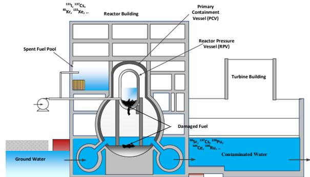
Fig. 5. Release pathways to the contaminated water.
