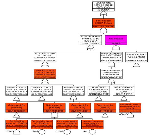
Fig. 2 Detailed Fault Tree of LODCA IE after modification
