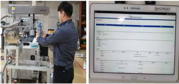
Fig. 3. QR code scan with a Smart-Pad, Equipment Information on Smart Pad.
