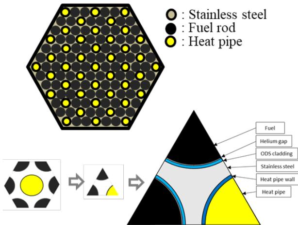
Fig. 7. Minimum cut of 'design 1' sub-channel of H-MMR
