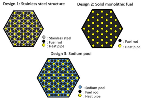
Fig. 6. Fuel assembly design of H-MMR core using heat pipe
