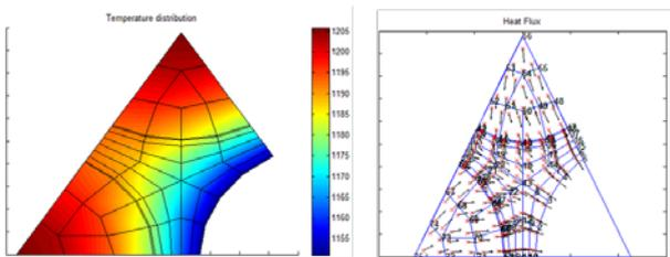
Fig. 8. FEM sub-channel analysis of 'design 1' of H-MMR
