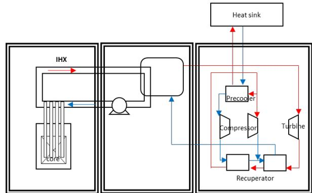
Fig. 5. Schematic diagram of H-MMR heat transport system
