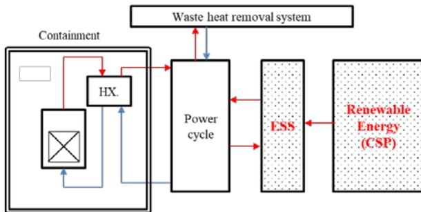
Fig. 1. Conceptual view of nuclear and renewable hybrid MMR
