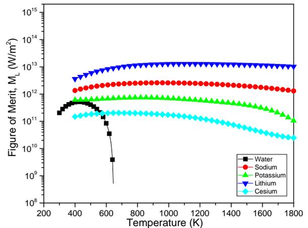
Fig. 2. Figure of merit (FOM) of heat pipe
