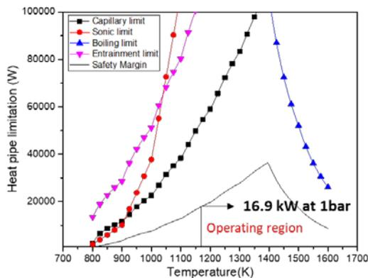
Fig. 4. Operating limits of the heat pipe in the annular gap wick
