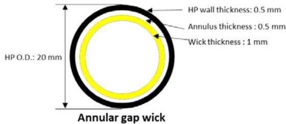
Fig. 3. Annular wick structure of capillary wicked heat pipe
