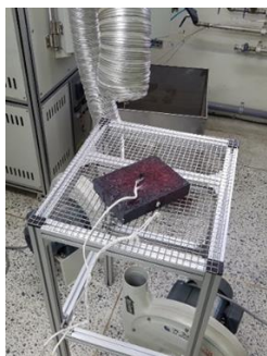
Figure 1. (b) Modified cooling method (Air Quenching, AQ)
