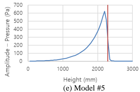
Fig. 3 Pressure amplitude of the initial model around the first mode natural frequency according to height. The red line indicates free surface height in each model.
