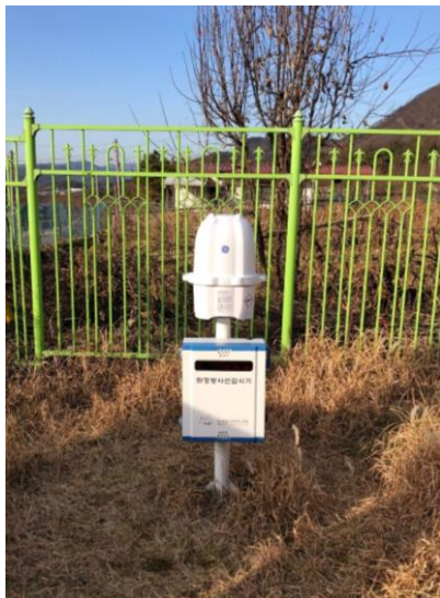
Fig. 1. Environmental Radiation Monitor deployed on site
