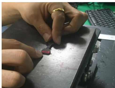
Fig. 5. Simulation with red guide beam before actual marking.
