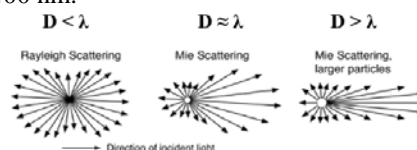
Fig. 1. Schematic illustration of Rayleigh scattering and Mie scattering
