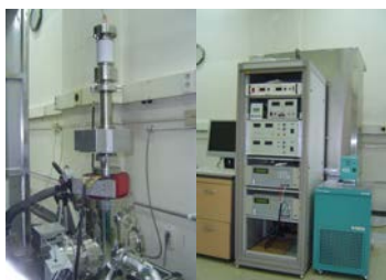
Fig. 2. Electron beam generator used in this work.
