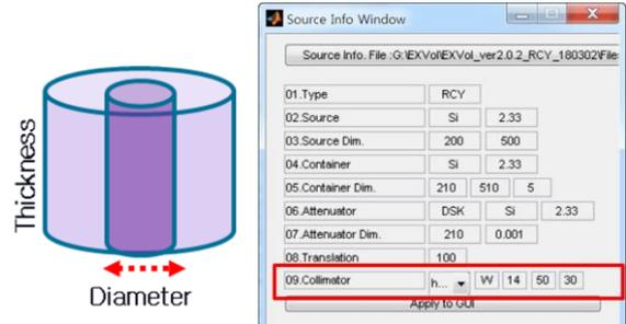
Fig. 2. Definition of a collimator and input value in the EXVol code.
