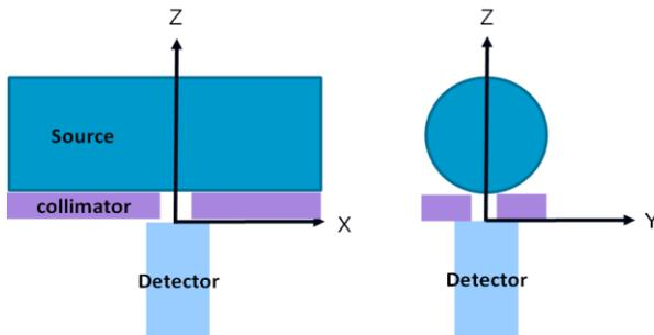
Fig. 1. Coordinate system of horizontal geometry.
