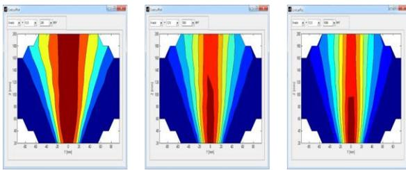
Fig. 5. Calculation results according to g-ray energy. 200, 500 and 1500 keV respectively (From left to right)
