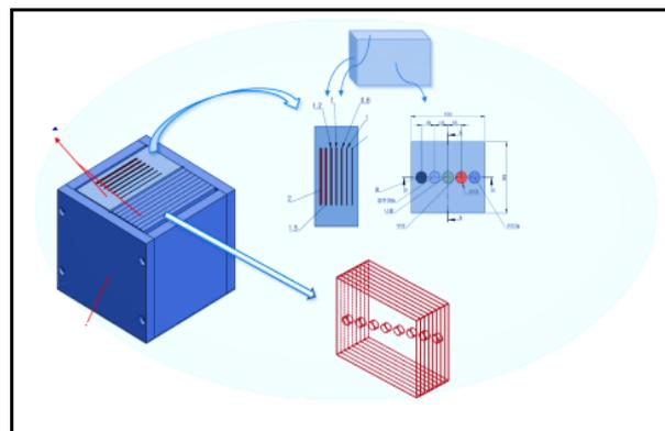
Figure 2 Drawing of a mixture of high (steel box) and low Z materials (PE plates) to be used as test sample for fast-neutron tomography
