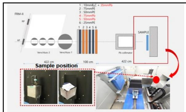
Figure 1 A collimator geometry for fast-neutron imaging at the NECTAR
