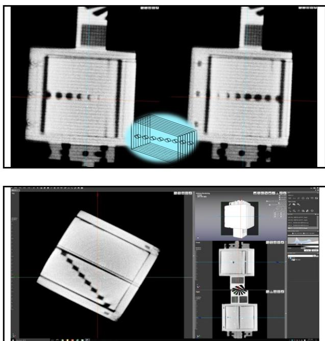
Figure 3 Fast-neutron tomography for the steel box filled with PE plates at the NECTAR
