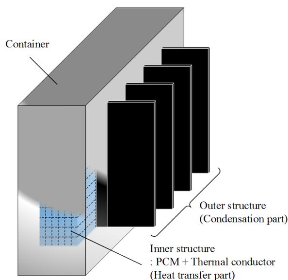
Fig. 2. Conceptual Design of PCM steam condenser module
