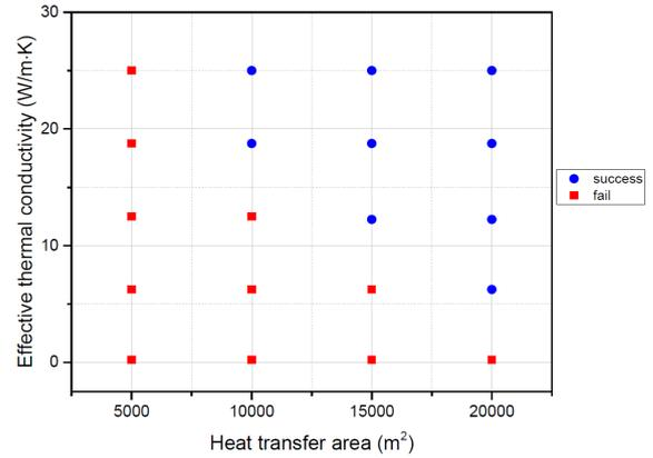
Fig. 7 Requirements for P58X PCM condenser for PCCS criteria
