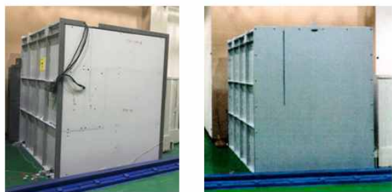
Figure 1. Neutron collimator made of polyethylene (left) and installed collimator (right)
