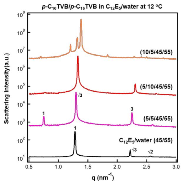
Fig. 2. SAXS intensities of  $\text{C}_{12}\text{E}_5/\text{water}$  (45/55) and  $p\text{-C}_{10}\text{TVB}/p\text{-C}_{16}\text{TVB}/\text{C}_{12}\text{E}_5/\text{water}$  with different mixing ratios at  $12^\circ\text{C}$ . Scattering intensities are shifted vertically for visual clarity.
