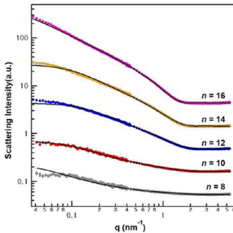
Fig. 1. SANS intensities of 0.1 wt %  $p\text{-C}_n\text{TVB}$  in  $\text{D}_2\text{O}$  for  $n = 8, 10, 12, 14,$  and  $16$  (color line).  $10\text{mM NaCl}$  is dissolved in  $\text{D}_2\text{O}$  to minimize electrostatic interaction between  $p\text{-C}_n\text{TVBs}$ . The black lines are model fits using a cylindrical particle form factor. The SANS intensities are shifted vertically for visual clarity.
