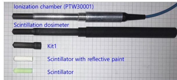
Fig. 1. Photograph of the ionization chamber, the scintillation dosimeter and its components.
