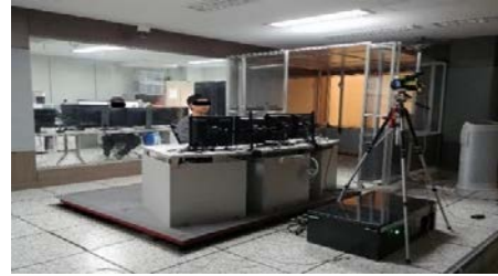
Fig. 2. Nuclear Power Plant Main Control Room Earthquake Simulator in the KAERI
