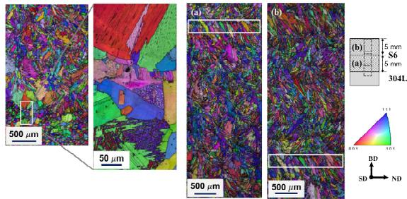
Fig. 2. EBSD map of AM Stellite 6 alloy on 304L stainless steel base plate, demonstrating the structure, size distribution and the orientation of the grains.
