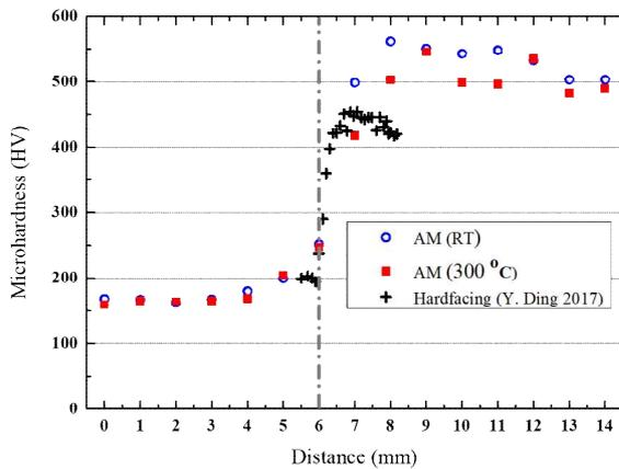
Fig. 3. Microhardness of AM cobalt-base Stellite 6 deposition layer compared with that of hard-faced one [3].
