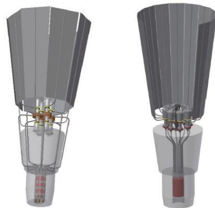
Fig. 2. Concept of Kilopower with sodium heat pipe [6]
