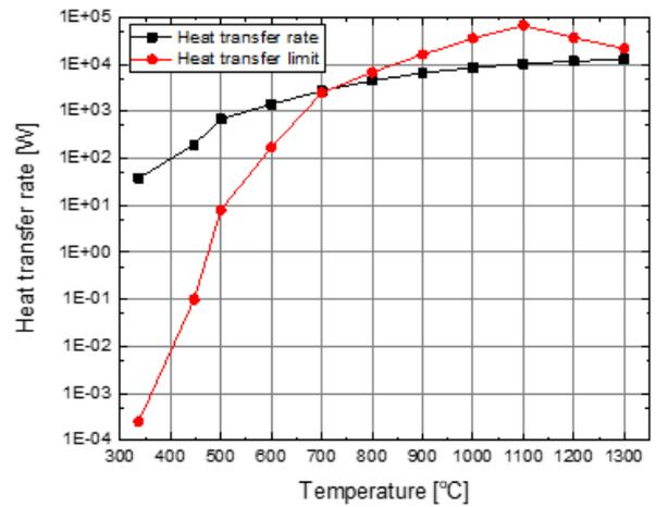
Fig. 8. Comparison between heat transfer limits and heat transfer rate according to operation temperature.
