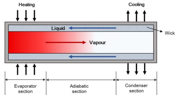
Fig. 1. Structure of heat pipe.
