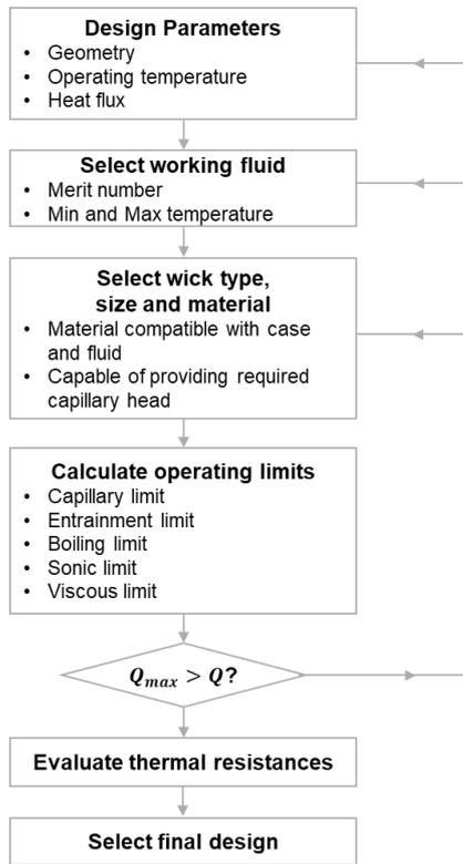
Fig. 3. The design procedure for a heat pipe [7].
