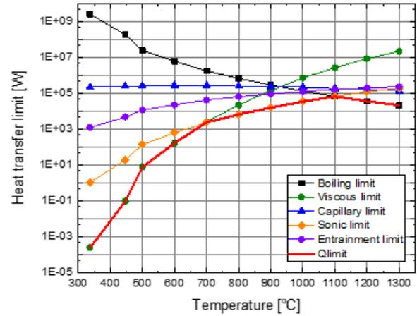
Fig. 7. Results of various heat transfer limits according to operating temperature.
