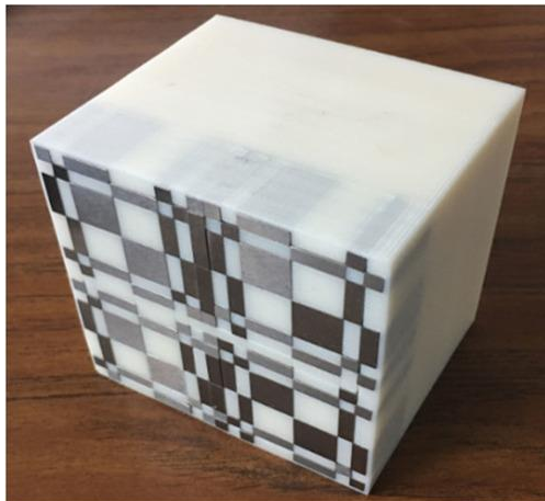
MURA mask fabricated with a 3D printer and 20 mm thick tungsten pieces
