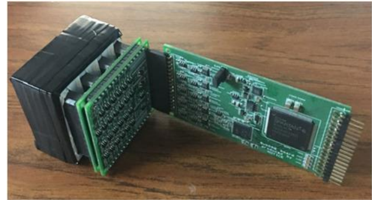
Detector system including DAQ board
