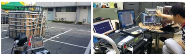
Fig. 6. Water tank for measuring the neutron-induced gamma test (a) and developed system for measuring of neutron-induced gamma spectrum (b).
