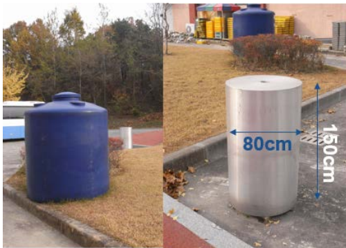
Fig. 3. Density sonde calibrators. The left is a water tank with a density of 1.0 g/cm 3 and the right is an aluminum block with a density of 2.7 g/cm 3 .
